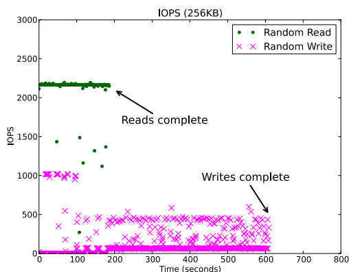
(b) Using RAILS to separate reads from writes across drives nearly eliminates the interference of writes on reads.
