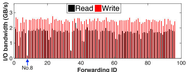
Figure 5: Forwarding node peak performance. Forwarding nodes with IDs 3, 8 and 34 show abnormal performance.
