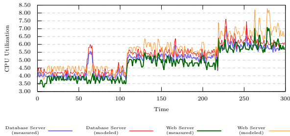
Figure 3: The CPU utilization for the marketing scenario; the model is not synchronized with observed measurements.
