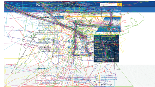
Figure 8: A visualization of the gaze of all users when viewing fcc.gov . Certain regions on the page have more gaze fixations than others (as evidenced by the thicker lines).
