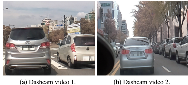
Figure 3: Videos recorded by our ViewMap-enabled dashcams that perform license plate blurring in real time.
