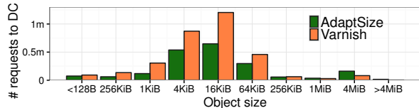
Figure 16: Comparison of the distribution of request sizes to the disk cache under a HOC running AdaptSize versus unmodified Varnish. All object sizes below 256 KiB are significantly less frequent under AdaptSize, whereas larger objects are slightly more frequent.
