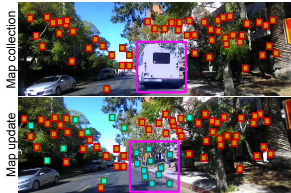
Figure 7: When adding a new region to the base map, the vehicle uploads the whole map segment (above). For updating an existing map segment, CarMap generates a map diff containing new map features (below, new map features marked in blue).
