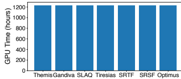
Figure 11: [TESTBED] Comparison of total GPU times across schemes with Workload 1. Lower GPU time indicates better utilization of the GPU cluster
