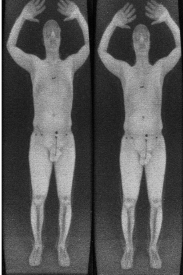
Figure 6: Concealing Explosives by Shaping — Left: Subject with no contraband. Right: Subject with more than 200 g of C-4 plastic explosive simulant plus detonator, molded to stomach.
