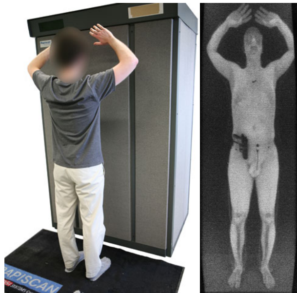
Figure 1: The Rapiscan Secure 1000 full-body scanner uses backscattered X-rays to construct an image through clothing. Naïvely hidden contraband, such as the handgun tucked into this subject’s waistband, is readily visible to the device operator.
