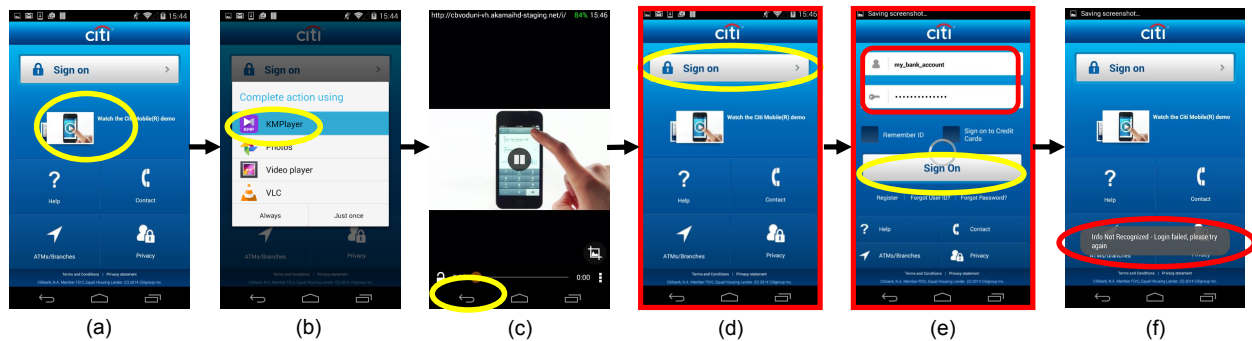
Figure 5: The process of “back hijacking” phishing attack to a well-known bank app. (a) shows the main activity of the bank app. A new user taps on the tutorial video link in the bank app; In (b), a system dialog prompts the user to choose a video player available in the system; In (c), the video player activity is started, and the user later clicks “back” button, intending to “goes back” to the original main activity; In (d) and (e), the back button directs the user to the phishing UIs, which spoof the user and steal bank account credentials. The phishing activity then quits after user clicks “Sign On”; In (f), the original main activity is resumed, with a log-in failure toast message displayed by the quitting malware.
