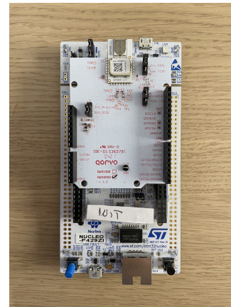
Figure 1: Shows a NUCLEO-F429ZI with the DWM3000EVB attached.
